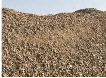
Dirty ballast at ballast depot
