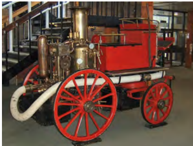
Preserved British steam-powered fire engine – an example of a mobile steam engine. This is a horse-drawn vehicle: the steam engine drives the water pump
